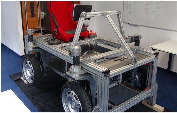
Fig. 1: fortiss eCar demonstrator - an experimental platform for innovative car architectures.
