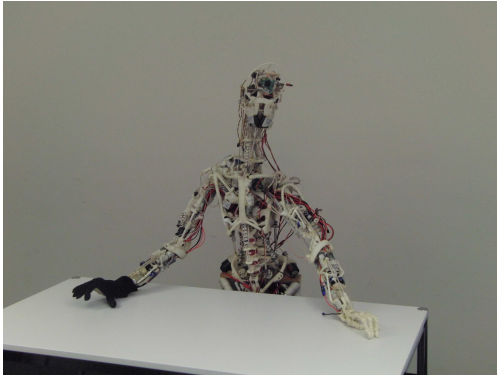
Fig. 1: ECCE1 – the first prototype of the ECCEROBOT series of anthropomorphic robots.
