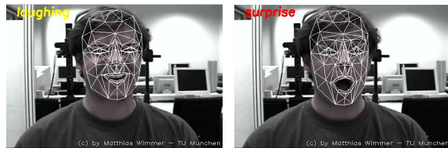
Fig. 4. The Candide-3 face model consists of 116 landmarks and reflects the face shape by 79 shape parameters.
