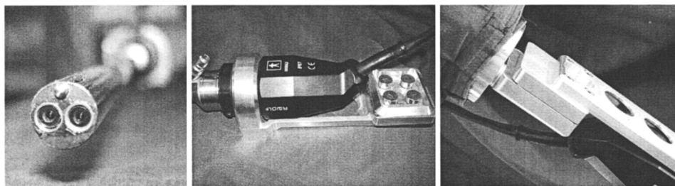
Figure 5. Endoscopic stereo camera with customized magnetic adapter.
