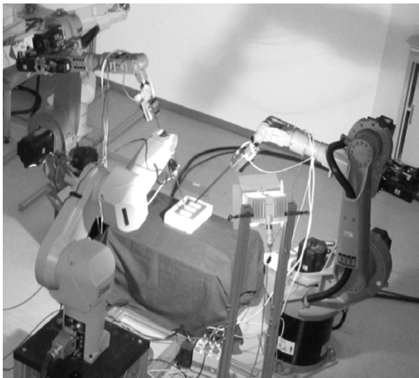
Fig. 1: Experimental robotic platform with integrated haptic feedback
