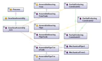
Fig. 4: Process model for the 3-step assembly of the core part of a gearbox. Boxes featuring a *yellow* circle or a *purple* rhombus represent classes and instances of those classes respectively.
