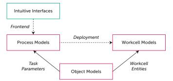
Fig. 2: Overview of semantic models and interrelations. Object models may serve as parameters for certain tasks specified in process models. A workcell model relies on object models for describing its entities. In order to execute process models, they are deployed on workcells using the information in their workcell models. Intuitive interfaces serve as a frontend to the semantic process models.
