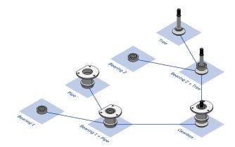
Fig. 5: Industrial use case based on assembling four work pieces in three steps to form the core part of a gearbox
