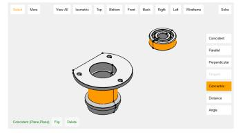
Fig. 9: Mode of the intuitive teaching interface for defining geometric constraints between two objects. As the two objects are described in a boundary representation, each of the two highlighted cylindrical surfaces can be selected with a single click. Geometric constraints can be chosen from the list on the right. A *PlanePlaneCoincidenceConstraint* (Fig. 6) has already been specified and is visualized in the bottom left corner of the GUI.
