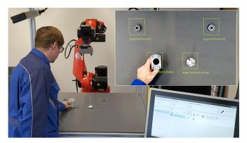
Fig. 1: Cognitive robotic workcell with features such as object recognition, projector-based highlighting, hand and body gesture recognition, and touch-based graphical interface for the task-level instruction of the robot.
