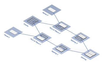
Fig. 10: Industrial use case based on assembling a frame and two wooden panels in five steps to build a wall of a wooden house. Different types of tasks are involved, i.e., pick and place, nailing, and sawing.
