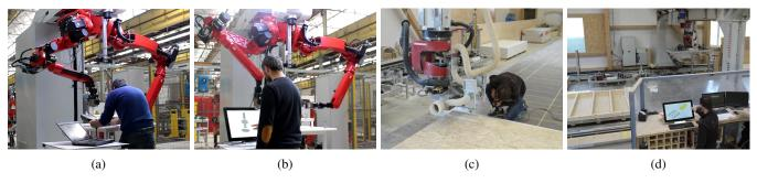
Fig. 11: Toward efficient robot programming: moving from (a,c) a classical approach using the teach pendant using low-level programming languages to (b,d) efficient robot programming using high-level semantic process descriptions.
